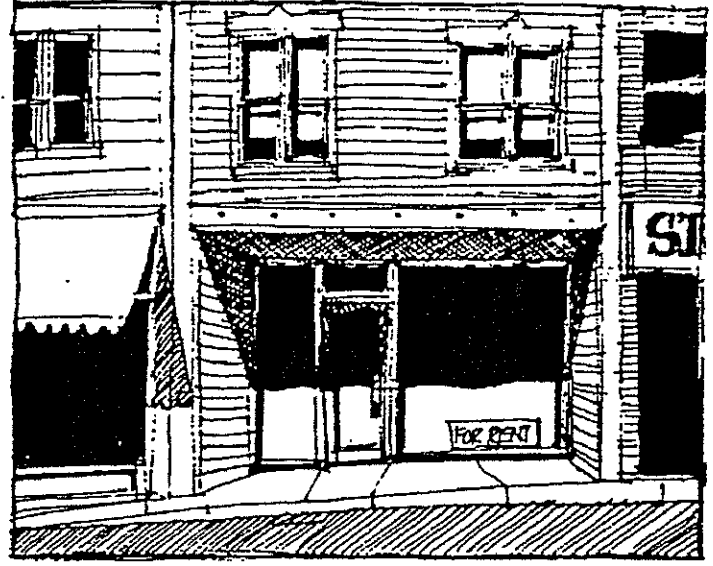
INAPPROPRIATE: ORIGINAL STOREFRONT COMPONENTS REMOVED
