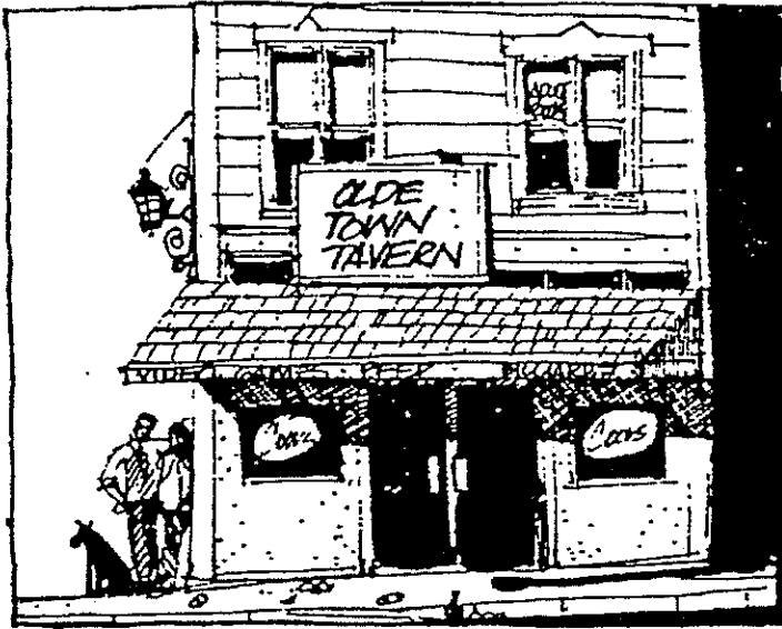
INAPPROPRIATE PORTIONS OF THE ORIGINAL FACADE CONCEALED
